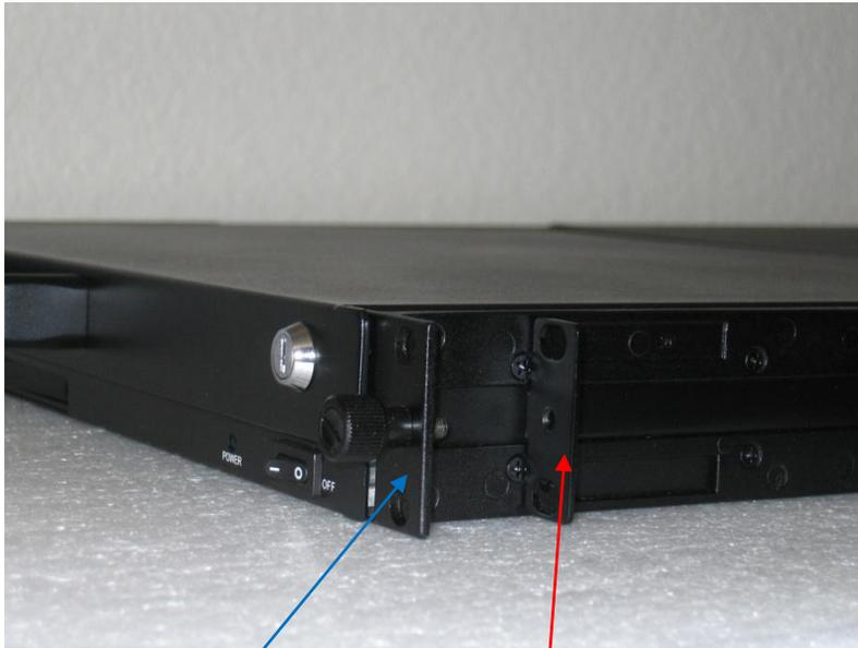
(1) First step: Unscrew the two thumbscrews on the front of Console and separate the two brackets as picture shows.
